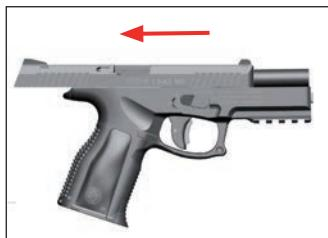
1. Pull back slide and pull down slide lock.
