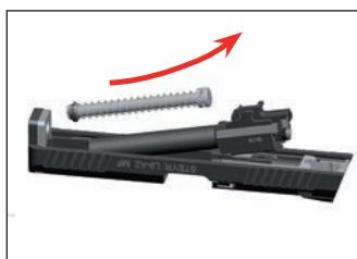
3. Remove the recoil spring and guide.
